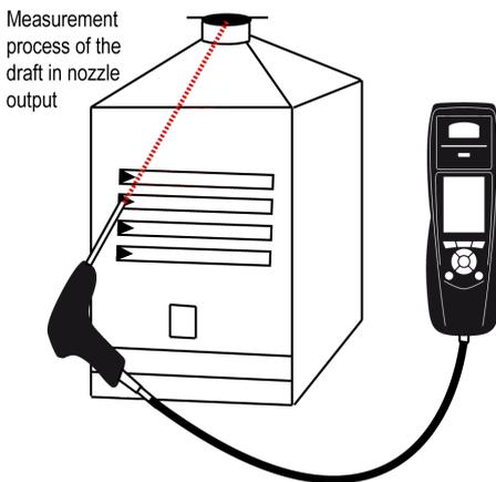
Put the probe of the KIGAZ 210 in the draft hood, going through the front face of the boiler
