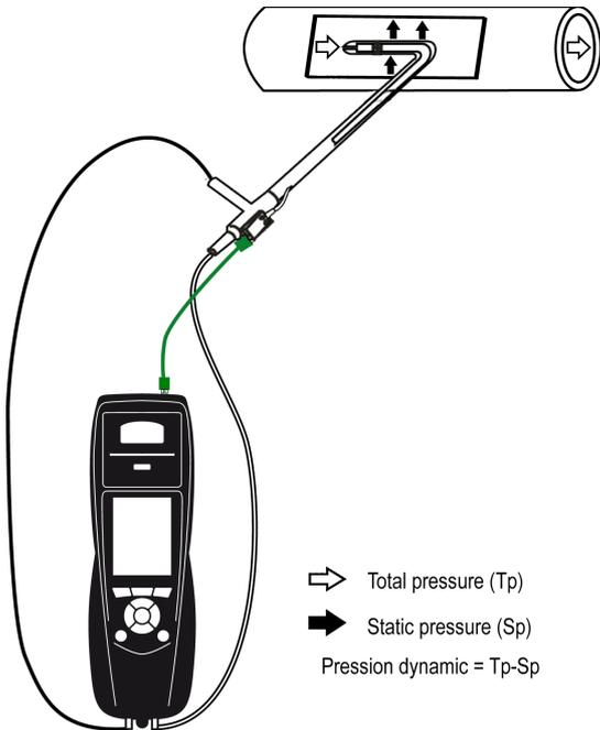
The Pitot tube must be introduced perpendicularly, in the middle into the duct and parallel to the flow.
