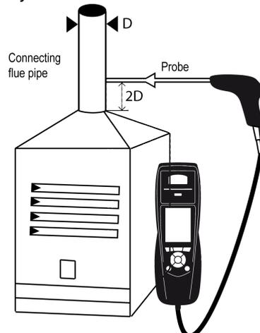
Put the probe of the KIGAZ 210 in the nozzle output, from the beginning of the connecting flue
