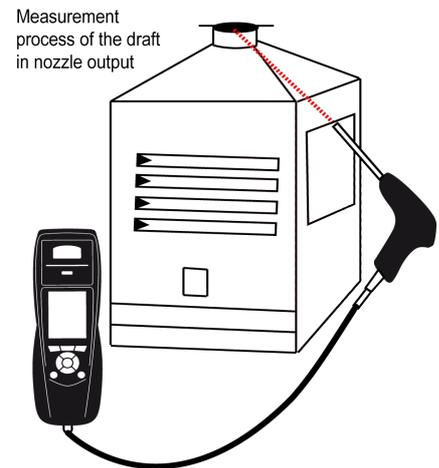
Put the probe of the KIGAZ 210 in the draft hood, going through the side openings of the boiler
